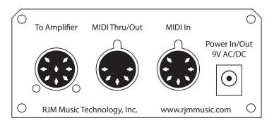
**To Amplifier** – Connect your custom amplifier interface cable here. Use the cable end that has a yellow label reading "Rack Gizmo / Amp Gizmo." The other end of the cable plugs into your amp's footswitch jack. Before connecting, make sure that you have the cable that's made specifically for your amp, or the ¼" adapter cable if your amp has ¼" footswitch jack(s). Cables are available for a variety of amplifiers. Check our website for a list of currently available cables.
