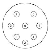
The Mini Amp Gizmo amplifier connector is a female DIN-8 jack. When a switch is activated on the Mini Amp Gizmo, the corresponding pin is shorted to the connector's ground (shield). Activating Switch 1 shorts pin 1 (as numbered above) to the connector's ground. Activating Switch 2 shorts pin 2, and so on.
